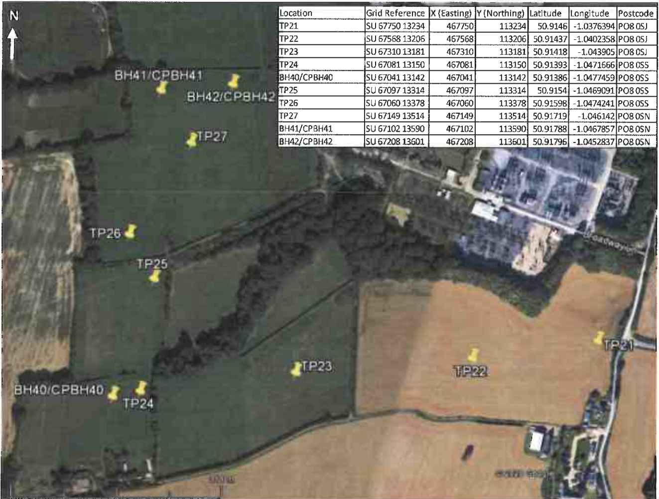
Figure 1 Converter Station Infiltration Testing Plan
